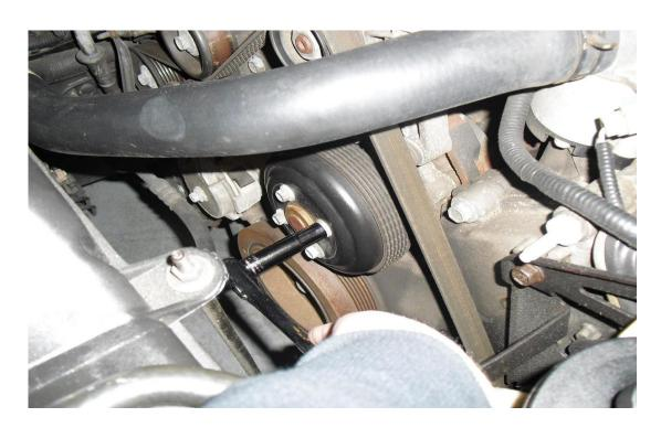
2. Loosen crankshaft balancer by using a 1/2" drive breaker bar and an 18mm socket. **Tip:** For manual transmission cars, place car in gear before loosening crank bolt. For automatic transmission cars, remove transmission inspection cover and wedge a wrench in between the **flywheel** and bell housing to prevent the engine from turning over.
