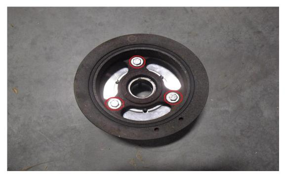
6. Place high-temp RTV silicone into keyway on pulley assembly and slide onto crankshaft snout as shown. Install new supplied crankshaft bolt with factory washer and tighten to 60 ft-lb. using a torque wrench.
