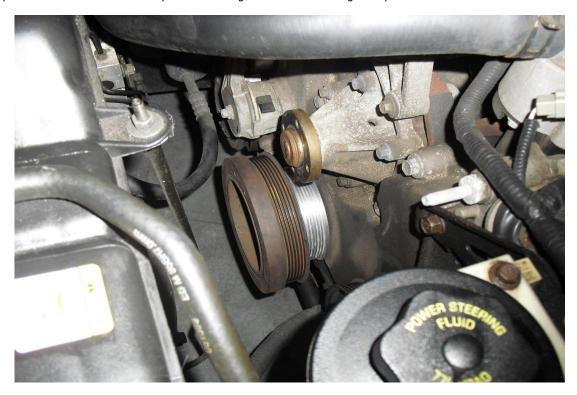
7. Using factory nut, install new alternator pulley with an impact gun. Using factory hardware, install new water pump pulley with a ratchet and 10mm wrench.
