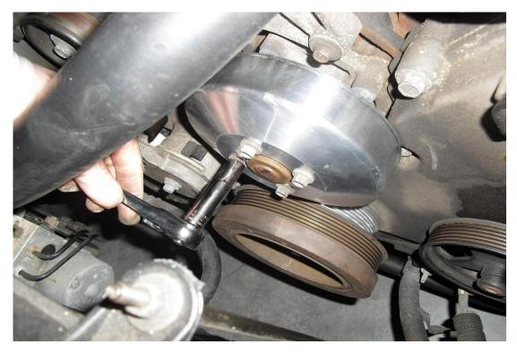
8. Re-install accessory drive belt and re-connect battery to complete installation. When restarting vehicle, make sure the pulleys are properly aligned and there are no unusual sounds before taking the car for a drive.
