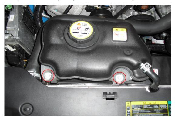
3. Remove the fan shroud be removing the 8mm and 10mm bolts securing it to the radiator. On the driver side, it is located just under the hose leading to the overflow bottle. On the passenger side, it is located just under the upper radiator hose.
