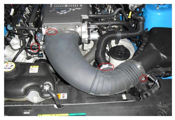
2. Remove factory coolant overflow bottle by removing the 8mm bolt and 10mm bolts holding it to the fan shroud.
