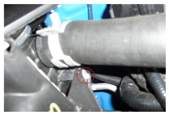
4. Loosen the four water pump pulley bolts using a ratchet and 10mm socket.
