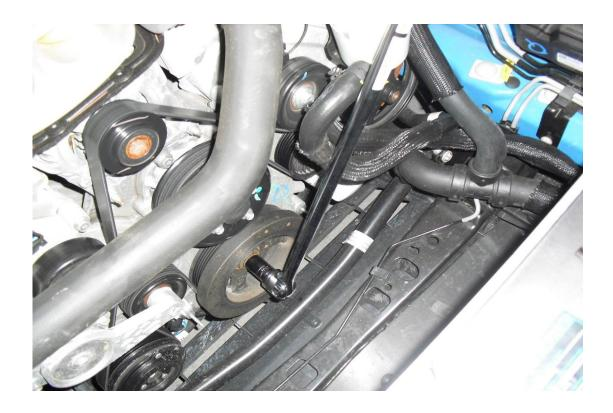
6. Once the crank bolt has been loosened, use a 1/2" drive ratchet to remove the accessory drive belt.
