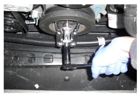
8. Make sure crankshaft snout is clean before installing new balancer. Apply a light bead of high-temp RTV silicone to keyway on Stack Racing balancer, then slide balancer onto crankshaft snout. The balancer will not be fully seated at this point, follow instructions in Step 9 closely to pull the balancer fully onto crankshaft snout.
