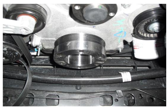
9. Using the supplied bolt and factory washer, tighten until the factory bolt can be safely threaded into the crankshaft snout. Do not over-tighten supplied bolt, it is only to be used to draw the balancer far enough onto the snout until the factory bolt and washer can safely be threaded into the snout. Once balancer is fully seated, use the following procedure to properly torque the bolt to Ford factory specs:
