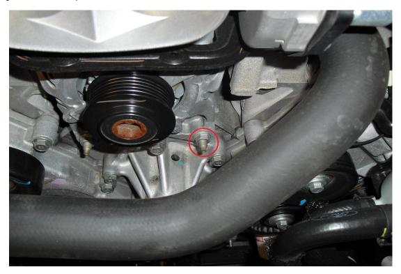
10. In order to make clearance for the new water pump pulley, you must grind down once of the water pump studs for clearance. You can either use a Dremel or Rotary Tool to cut the stud on the car, or you can remove and use a hacksaw. Shown below is the stud before and after trimming.
