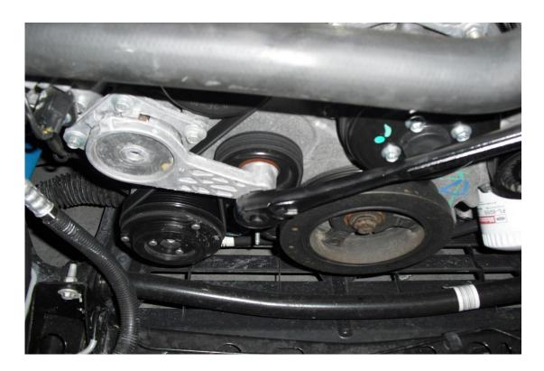
7. Once the belt has been removed, fully remove the factory crank bolt and washer. Re-thread the bolt without the washer about halfway into the crankshaft. Use a three prong pulley puller tool to remove factory balancer from crankshaft.
