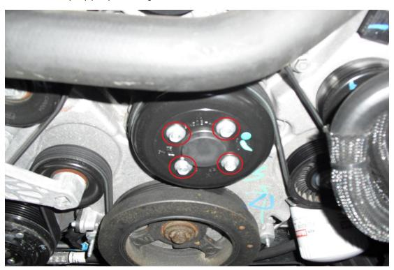
5. Using an 18mm socket and a breaker bar (or an impact gun), loosen the crankshaft bolt.
