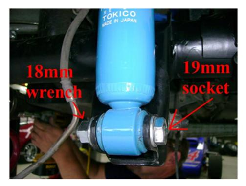
10. Before you put the top end of the shock through the hole, make sure that you have the lower washer and lower rubber pieces on the bolt.
