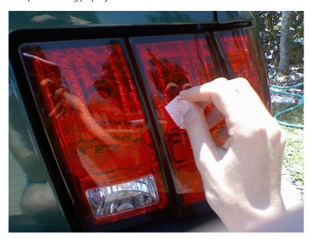
3. Remove the tabs from the double sided tape and align the tail light covers with the top-outside corner of the tail lights. Then, press the tail light covers onto the tail lights.
