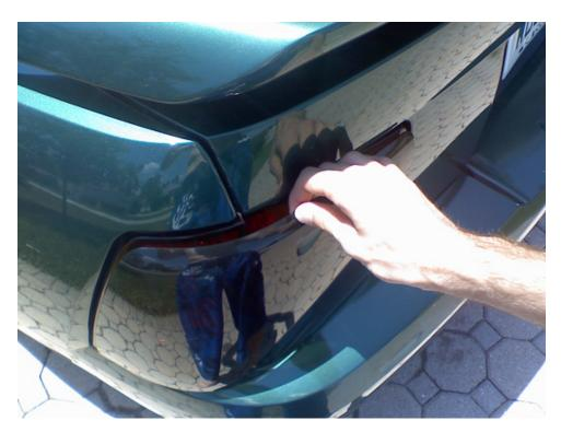
4. Quickly make sure the tail light covers are lined up the way you want them to be, because the double sided tape will quickly bond after a few seconds. If the edges don't look like the following picture, quickly remove them and try again.
