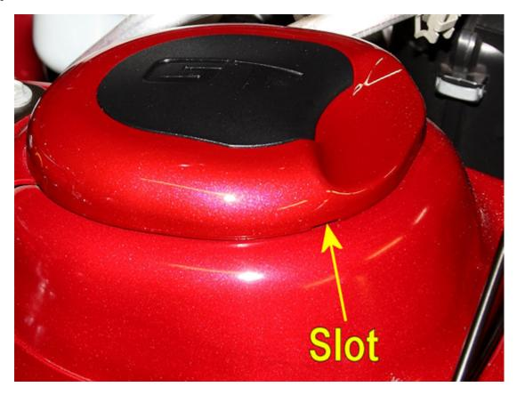
2. Insert a flathead screwdriver into the slot, and twist it to raise the shock tower cover up. Once you start to raise the cover, pull it the rest of the way off by hand.
