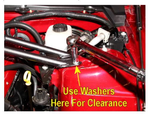
8. Recheck the clearance after you've tightened the strut brace down. You don't need huge amounts of clearance, as S197 Mustangs see much less engine movement than previous Mustangs. If you have a buddy have them watch the engine and brace, checking for clearance, as you rev the car a few times.
