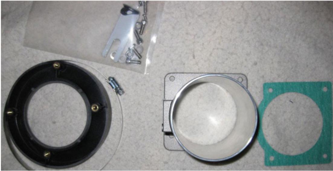
(Above) Circular-shaped air guide, (2) Small screws, (4) Medium screws with washers. Billet meter, Billet meter gasket, Large hose clamp.
