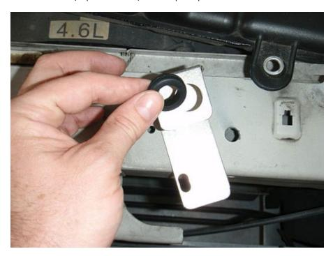
8. Now place the supplied stainless radiator brackets where the old brackets were. The bracket that is not completely straight is the driver side bracket. The straight bracket goes on the passenger side.
