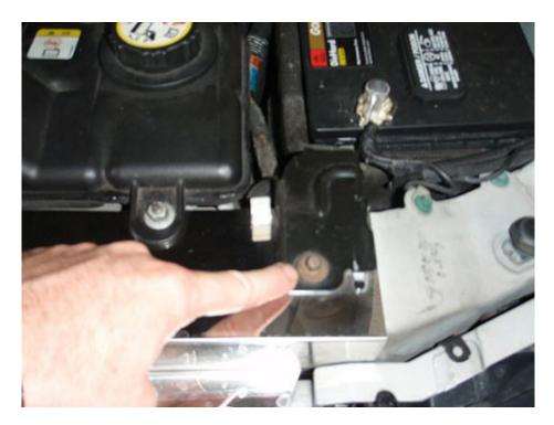
5. Then unscrew the radiator reservoir with an 11mm socket. There are two screws as pictured below.
