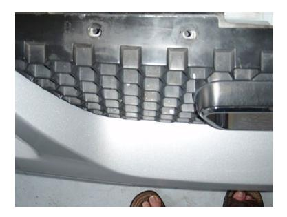
4. Next unscrew the driver and passenger side radiator brackets with the 8mm socket. Pictured below is the driver side.
