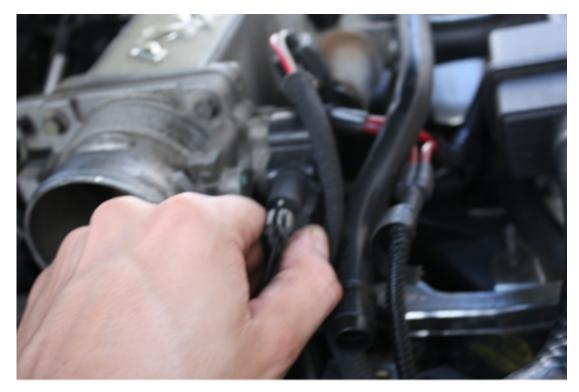
6. Remove the 4 bolts securing the throttle body to the plenum.
