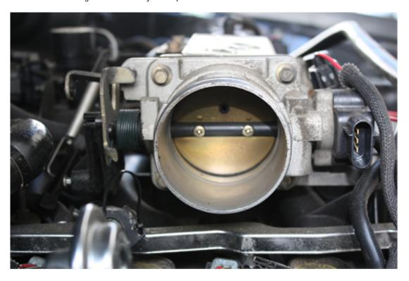
7. After you have removed the stock throttle body from the engine, remove the Throttle Position Sensor from the stock throttle body. This piece will have to be reused on your new throttle body. Take care in unscrewing the sensor, the screws will strip easily.
