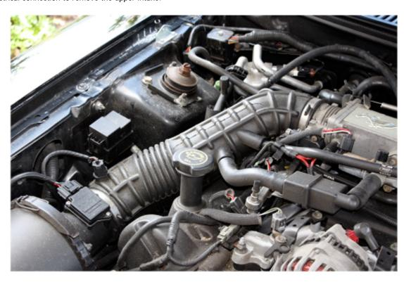
Remove the Throttle Cable, Cruise Control Cable and Throttle Body Spring from the left side of the throttle body. The throttle body spring simply unhooks from the throttle body. The Cruise Control Cable lifts straight "up" and pops off as pictured.
