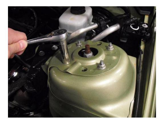
2. Place strut bar over strut mount studs and re-install 13mm nuts removed in Step 1.
