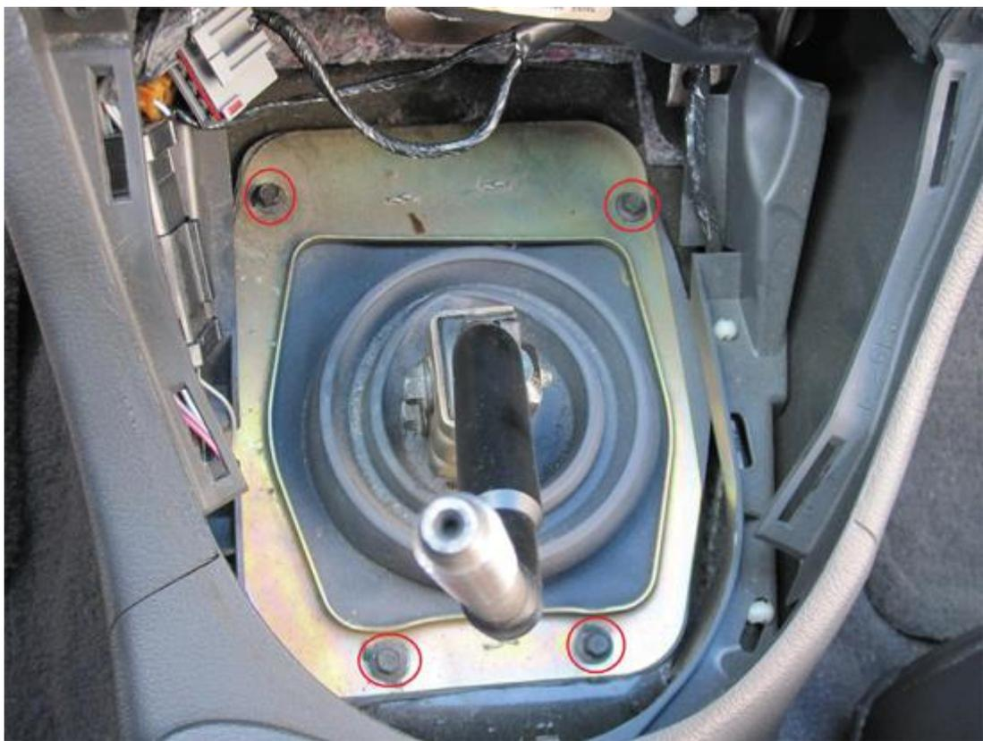
3. Lift up on the boot to expose the (4) 13mm nuts that hold the factory shifter to the transmission and remove them.
