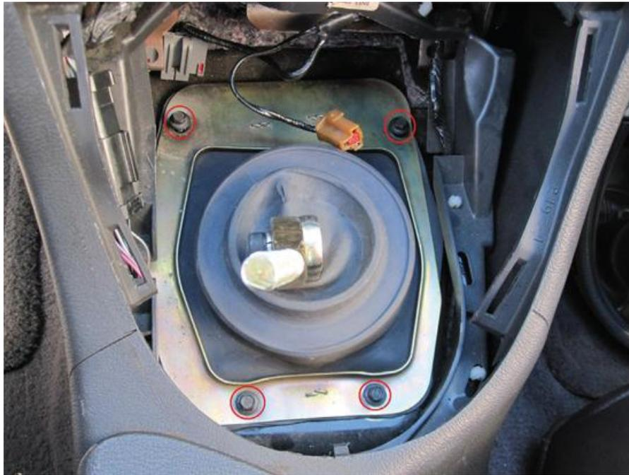
9. Re-install the factory shift bezel by pushing down on the clip and plug in any electrical harnesses that were disconnected in Step 1. Re-install your shift knob to complete the installation.
