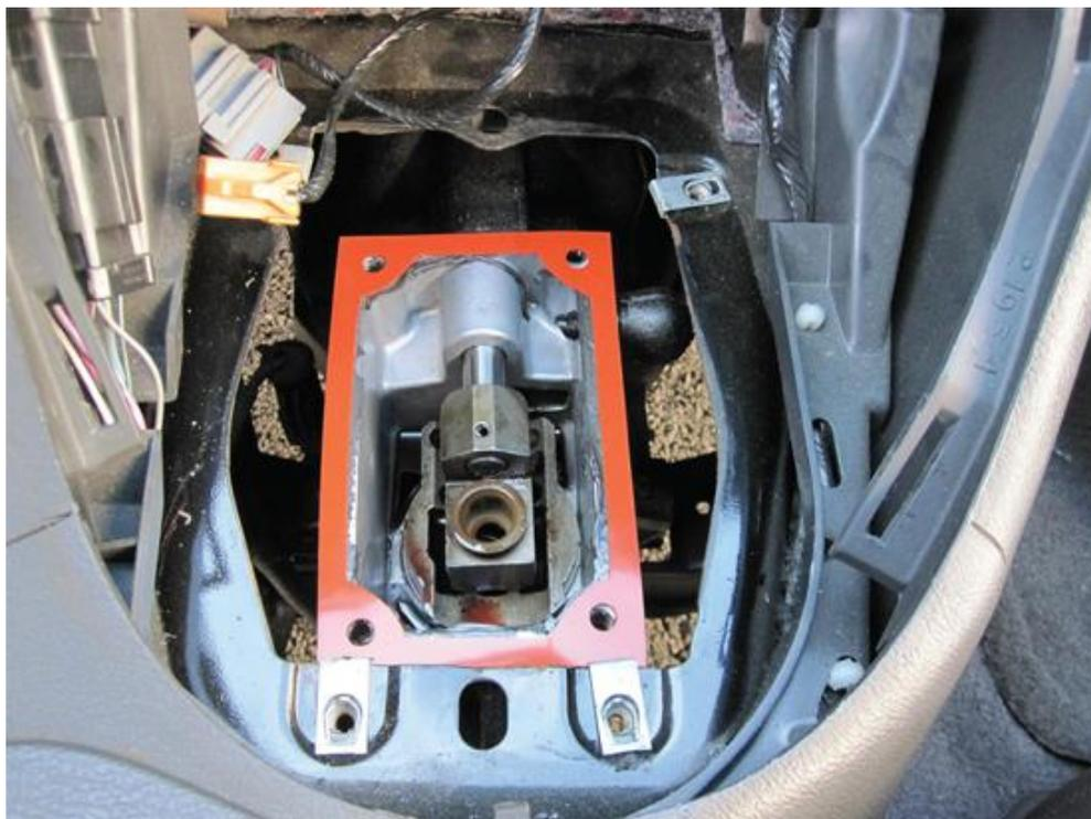
7. Place your new shifter assembly on top of the transmission and use the supplied 13mm bolts to secure it to the transmission. Adjust your shifter using the stop nuts and bolts so that the transmission goes freely and completely into all gears. Leave about  $\frac{1}{4}$ " between the stop bolt and the shifter when the shifter is fully engaged in each gear. The shifter should not hit the bolts during normal operation. They are there to prevent transmission damage under hard shifting.
