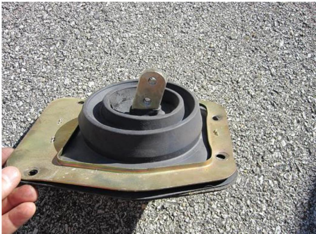
6. Scrape off any left over RTV left on the shifter housing of the transmission and install a new gasket or a thin bead of black RTV silicone.
