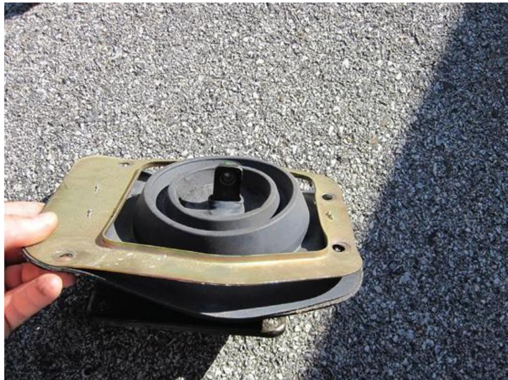
5. Using an allen key, remove the handle from your new shifter and slide the rubber boot over top of it as shown. Re-install the allen head bolts and tighten.
