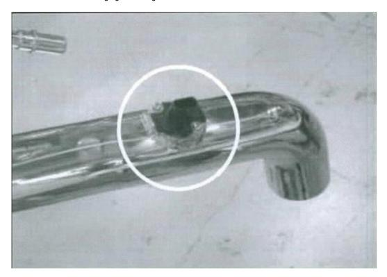
8. Install the supplied adapter hose onto the throttle body as shown using the hose clamp.
