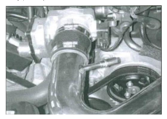
10. Attach the stock plastic breather hose by pushing it over the aluminum nipple on the intake pipe until it snaps into place.
