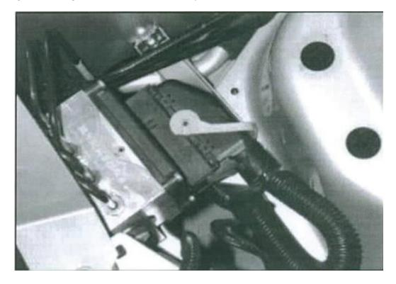
7. Check to be sure that the intake pipe is clear from debris. Install the MAF Sensor using the supplied mounting screws. Use Caution to avoid damaging the o-ring.
