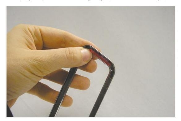
3. Once the backing tape is removed, carefully line the trim up with the outer edge of the light. Take care not to press down on the trim during this step.
