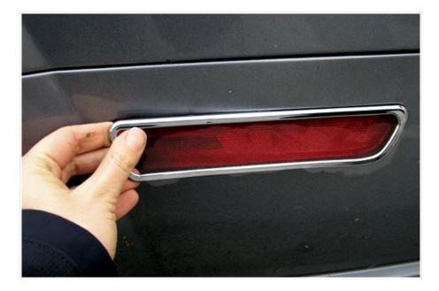
4. When you feel you have successfully lined the trim up with the grooves of the light, press firmly along the entire surface of the trim to ensure a complete and sturdy bond is made with your light.
