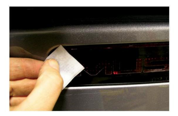
2. Before applying the trim, make sure all of the backing is completely removed from the 3M bonding tape .
