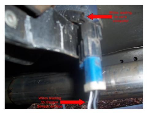
5. A blue (passenger side) or white (driver side) connector is attached to this. The four wires will run in a sheath to the Oxygen Sensor on the mid-pipe.
