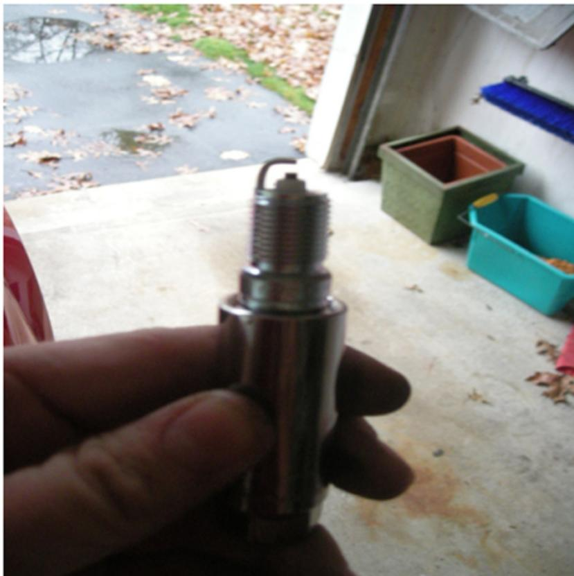
8. This step is a little tricky. Make sure the spark plugs stays in the socket, then you have to feel around and find the hole to insert the spark plug in. Once it is in turn it to the right (clockwise) by hand while pushing in until you cannot turn it anymore. Then attach your ratchet (using an extension if needed) and turn it until it is very tight.
