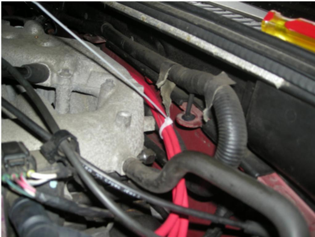
14. Once installed double check everything. Make sure all the plugs are secure and snug on the coil pack and spark plugs. If you removed your intake to make the install a little easier reinstall it now. Now start the car up. Make sure it idles smoothly and take it for a drive to ensure it runs smoothly as it should at all rpm's. If you start it up and something is wrong, turn the car off immediately and double check all your wires and connections.
