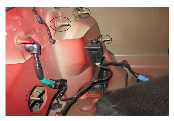
3. Once all of the nuts are removed, simply pull the tail light housing from the vehicle. Remove the <u>bulbs</u> by twisting them, making sure to take note of their position in the housing.
