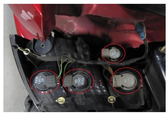
4. Install the bulbs in the new housing in the same position as they were removed from the old housing. Make sure to place the two wiring harness clips into the holes on the new housing to ensure the wires done get pinched upon reinstallation.
