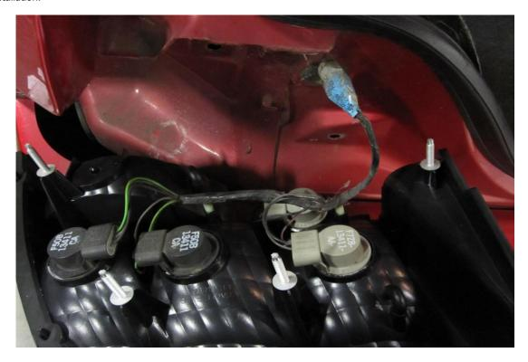
5. Place the housing back into the tail section of the vehicle and re-install using the 11mm nuts that were removed in Step 2. Repeat for other side then re-install any interior trunk trim that was removed in Step 1 to complete the installation.
