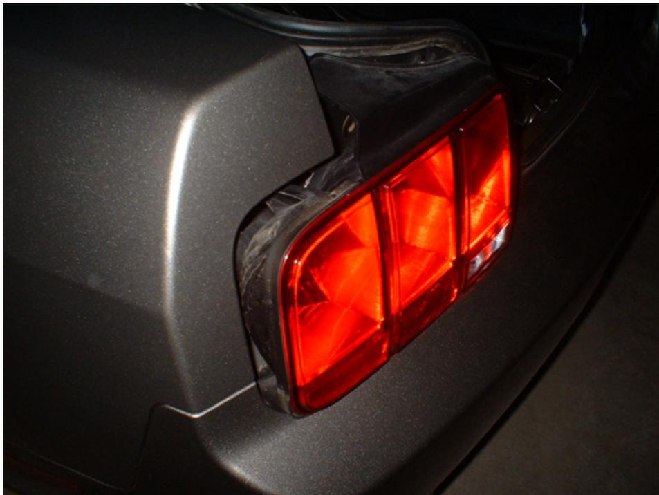
5. Transfer bulbs from old lights to new lights To remove the bulbs, turn them counter-clockwise (opposite the direction marked "Lock" on the bulbs). You may need to use an adjustable wrench or pliers to turn them. Be sure to retain the rubber washer on the back of the bulbs when you transfer them to the new housing. The bulbs will only fit into the housing one way, so make sure that they are aligned correctly when you re-install them.
