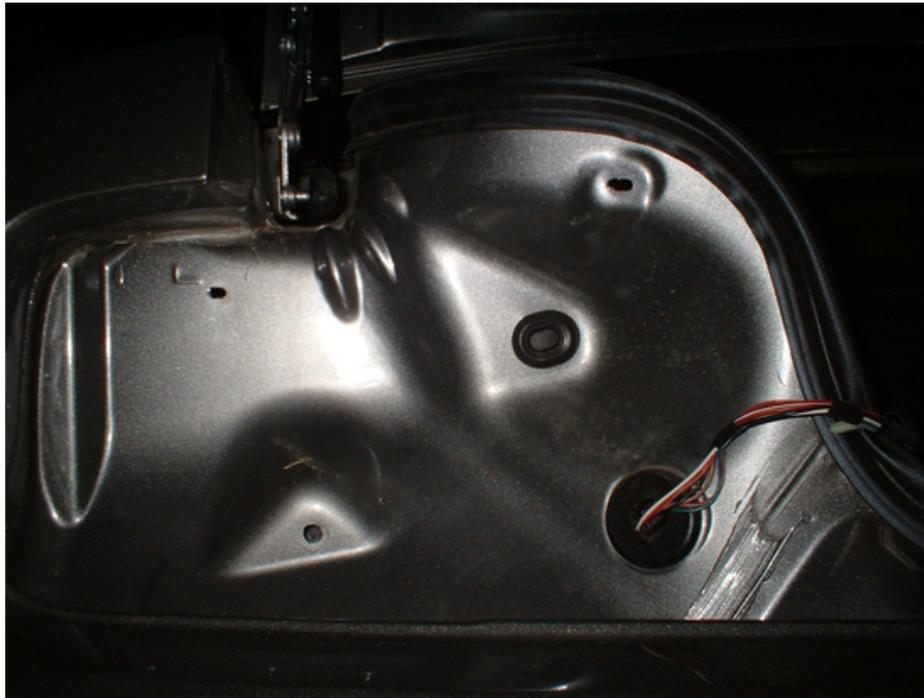
9. The final step is to replace the plastic cover on the inside of the trunk. When re-inserting the push fasteners, pull the center out before putting it through the hole (as shown in the picture above), then push the center piece down. The screw-type fasteners screw onto the end of the tail-light studs, so make sure everything is lined up properly. That's all. Put the spare tire cover back in the trunk, close the decklid, and wipe off the new tail-lights so they will be clean and shiny.
