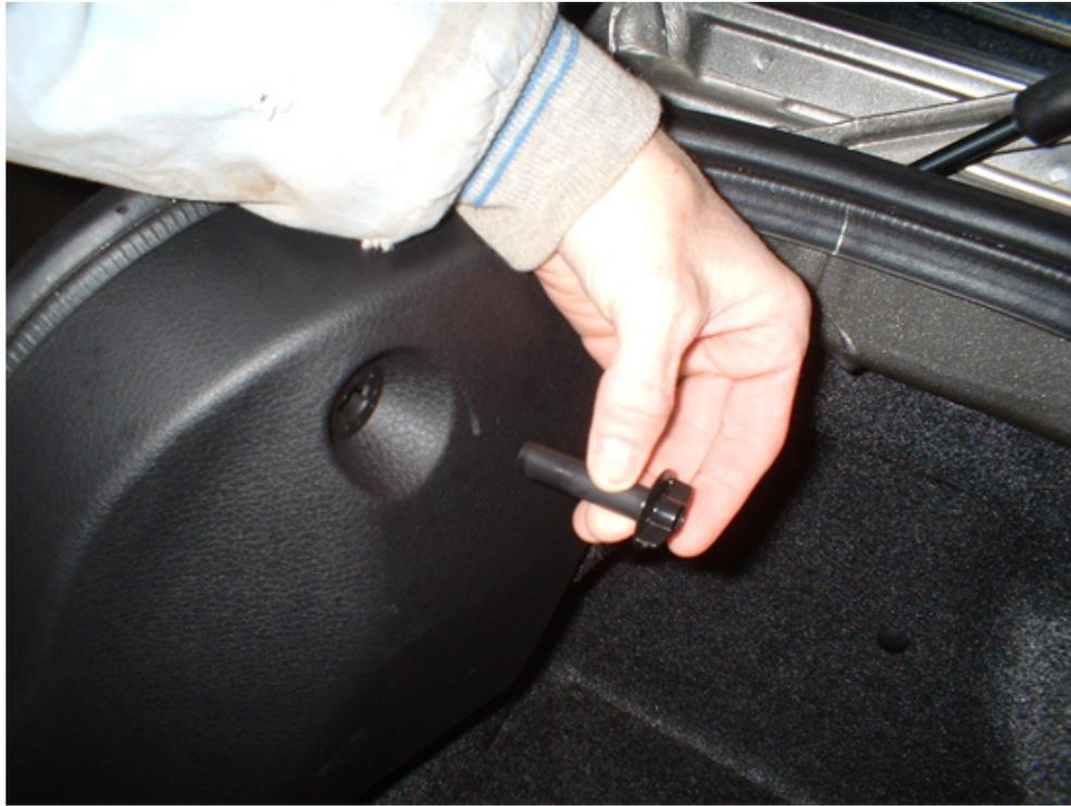
2. Use a screwdriver to pry up the center of the push-fasteners, then pull the fastener out. Once all the fasteners have been removed, lift the plastic cover out of the trunk.
