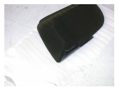
3. Grasping outside of new cover (avoid getting fingerprints on inside of covers) Angle the cover, starting at the bottom of existing headlight. Making sure that cover tucks inside of body panels, clip the cover to the top of headlight bezel and repeat with other side.
