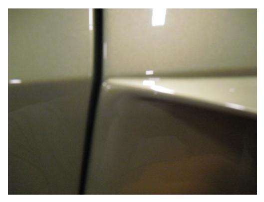
5. When certain that scoop is properly aligned, press down firmly where adhesive tape was applied to ensure a proper fit.
