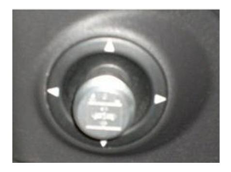
7. Test to ensure that the knob was installed properly by turning the knob to the left or right mirror adjustment position and attempt to adjust the mirrors. Once this is done, your installation is complete!
