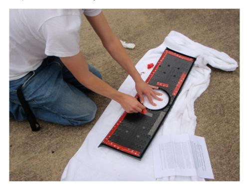
5. Have your assistant hold the panel open at a height that will allow you to work with it comfortably. Hold the panel a few inches away from the trunk lid and align the panel. If you hold your hands on left and right sides and apply pressure with your thumbs, the panel will flatten. This will allow you to place the center on first, followed by the sides.
