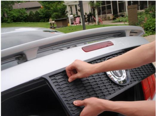
7. Allow for vehicle to remain at 60-80 F for at least one hour to aid in the adhesion of the tape. Do not wash the vehicle or let it get wet for at least 24 hours after installation.
