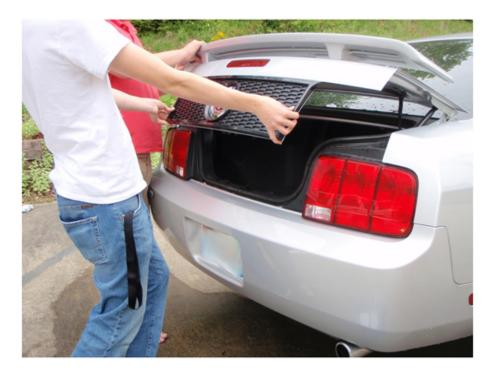
3. Place the panel on a soft surface for the moment and wipe the lid down with the alcohol wipe. Make sure the entire trunk lid (where the product is to be placed) is wiped down so all of the dust is removed.
