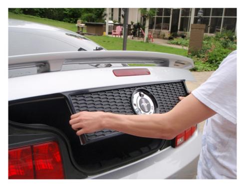
6. After installation, use firm hand pressure to push the panel/tape down onto the trunk for a minimum for 4-5 minutes. Work your way around the panel to achieve a uniform adhesion.
