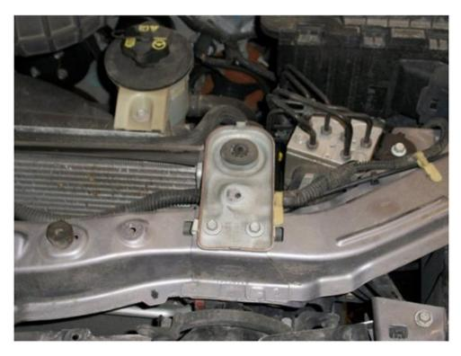
4. Install metal brackets underneath radiator support. Brackets must face towards outside of engine compartment, as shown here from the driver's side. Tighten bolts.
