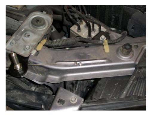
15. Route lanyard around brackets and place through corners of the grille. (Fig 8)
