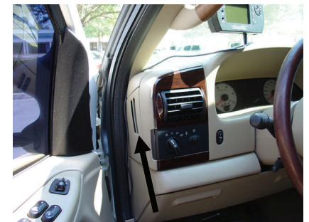
Route Cable Down The Side Of The Dash/Door
