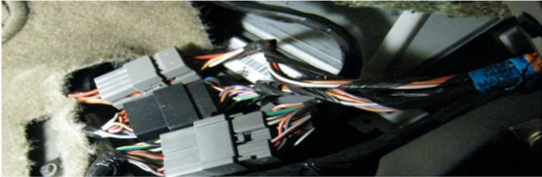
5. Next, you will have to take the 7mm Socket and remove the two bolts holding the bracket attached to the three connectors. After the bracket is free, you can now get your hands in towards the computer. Unscrew the one 10mm bolt on the bottom center of the computer and the one small golden 5.5mm bolt holding the plastic box that secures the computer.
