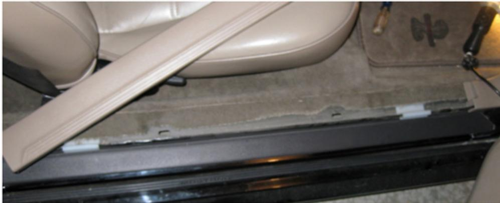
3. To remove the kick panel, just put your hand behind it and pull straight out on the tab. It comes right off.
