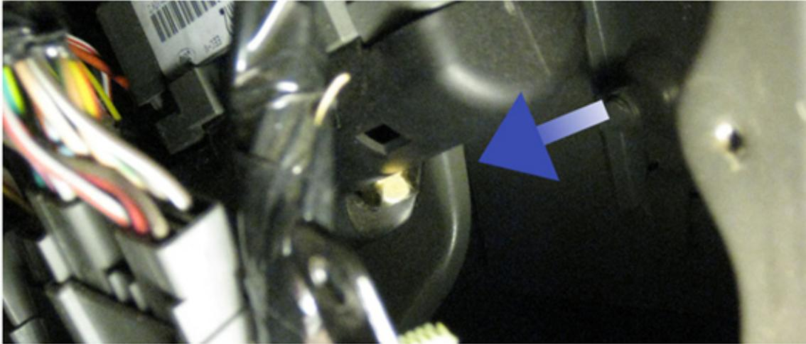
6. Once the bolts are removed, slide the computer out. The plastic covering of the J3 port needs to be removed. Take a screw driver or pliers, whatever you have around, and on the opposite side of where the computer was connected, gently slide this item under the tab to remove it.
