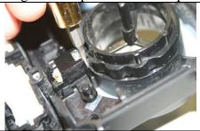
12. Install the new knobs, making sure they fully engage the back half of the knob assembly and snap into place. There is an index mark machined into the knob to correspond to the index mark on the back half of the assembly to aid in assembly – it is a small line, not completely cut through the back ring area. Check for free rotation throughout their intended range of motion, and then return them to the 12 o'clock position for re-assembly.
