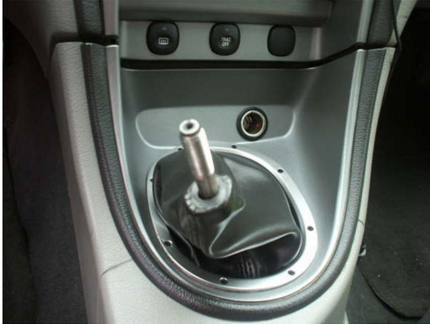
2. Thread on the supplied locking nut, turning it clockwise. The purpose of the nut is to lock your Roush Shift Knob tight, so it won't twist loose while your pony is winning a race. You are going to want the locking nut all the way down the threads of the shifter.
