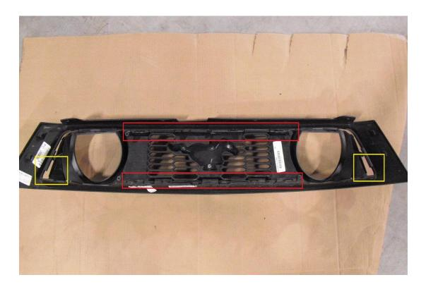
6. Place the billet **grille** inside of the outer factory grill shell. Once you have the desired location of the billet grille in the shell, use a drill and 3/16 bit to drill holes for the mounting hardware as shown.
