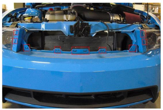
4. Remove the fog lights from the grille using a 7mm socket.
