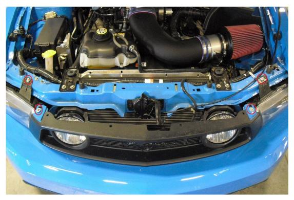
3. Use a flat-headed screwdriver to carefully pry the four outermost mounting tabs of the grille (two on each side) from the bumper cover. Once these outer tabs are loose, carefully but firmly pull up and out on the grille to fully release it from the bumper cover. Make sure to unplug the fog light wiring harness before completely removing grille from the vehicle. Use zip-ties to secure the harnesses to the radiator support as they will not be used after this install.
