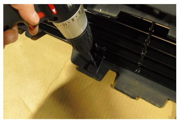
7. Once your mounting holes are drilled, place the four supplied U-nuts on the four mounting tabs of the grille and secure it to the outer factory grille shell using the four supplied screws as shown.
