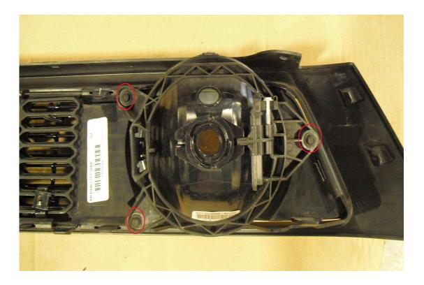
5. Remove the inner grille assembly from the outer grille assembly by first removing the corners of the grille (shown in yellow), and then by carefully prying the remaining mounting tabs (shown in red) with a flat-headed screwdriver.
