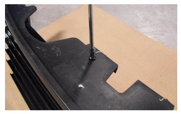
8. Once your billet grille is fastened securely to the outer factory grille shell, re-install the grille into the front bumper cover and reverse Steps 1-3 to complete installation.
