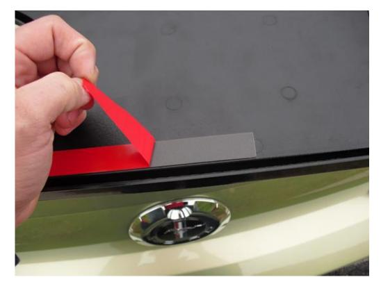
3. Place blackout panel over rear decklid using center pony emblem as a reference point. Make sure that blackout panel is centered and extends evenly to both sides of decklid. Also take care to ensure that corners meet top edge of decklid on both sides and follow contour of factory tail lights.
