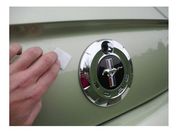
2. Peel the backing from the adhesive strips on the rear of the blackout panel.
