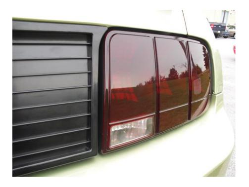
4. When blackout panel is properly aligned, firmly press down on adhesive strips to fully seat blackout panel.
