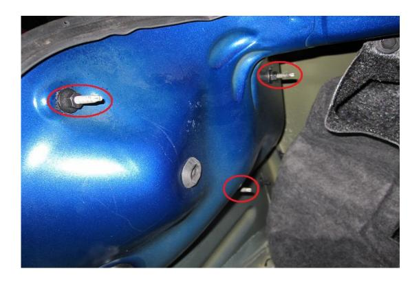
3. Remove the tail light housing from the vehicle and remove the bulb sockets by twisting them. Make sure to take note of each bulbs location so you can install them in the same order in the new housing.
