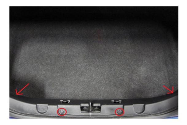
2. Use an 11mm socket or wrench to remove the 3 nuts holding the tail light to the vehicle.
