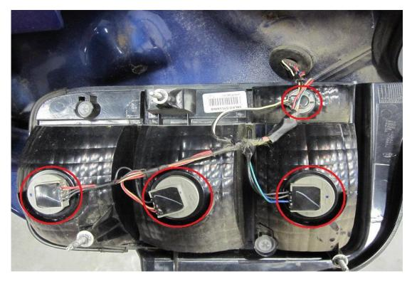
4. Place the bulbs in the new housing. The location of the reverse light bulb will change slightly if you are installing the 2010 style tail lights (shown below).
