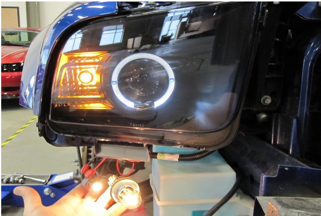
Driver Side: Red wire from new light – white w/ red stripe wire from parking light Black wire from new light – black wire from parking light
