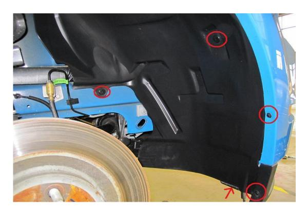
3. Remove the four 7mm sheet metal bolts holding the splash shield to the underside of the front bumper cover.
