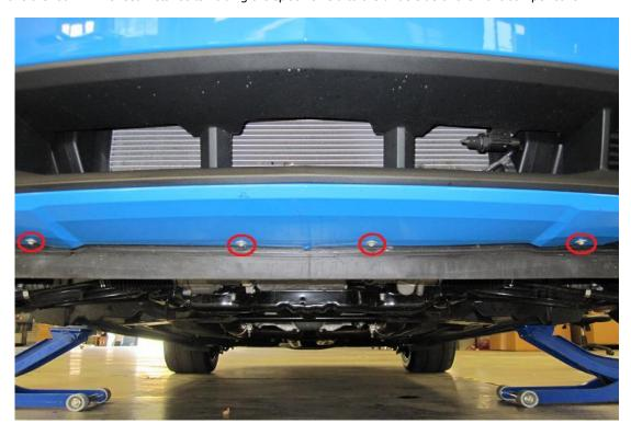
4. Remove the eight plastic retaining clips holding the plastic radiator cover on. Then remove the cover from the vehicle.
