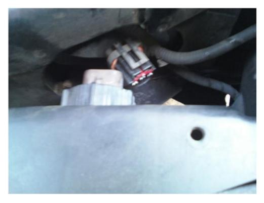
4. Now you need to remove the clip from the top bolt closest to the outside of the car. This can be done by prying on the clip with your flathead screwdriver.
