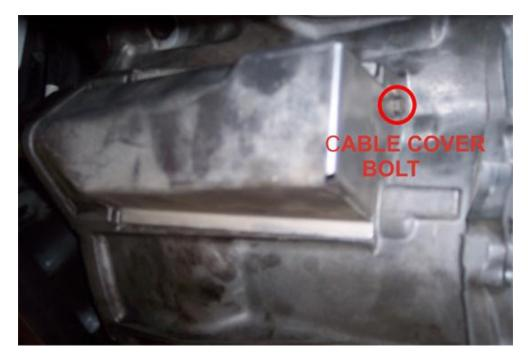
9. Next you will want to remove the starter. I found it easier to disconnect the electrical connections on the starter itself, using an extension I accessed the connections from the front. The you will need to remove the 3 (13mm) bolts holding the starter on. 2 bolts are clearly visible, the second is concealed. I had to feel around until I located the bolt, it is at the very top of the starter.
