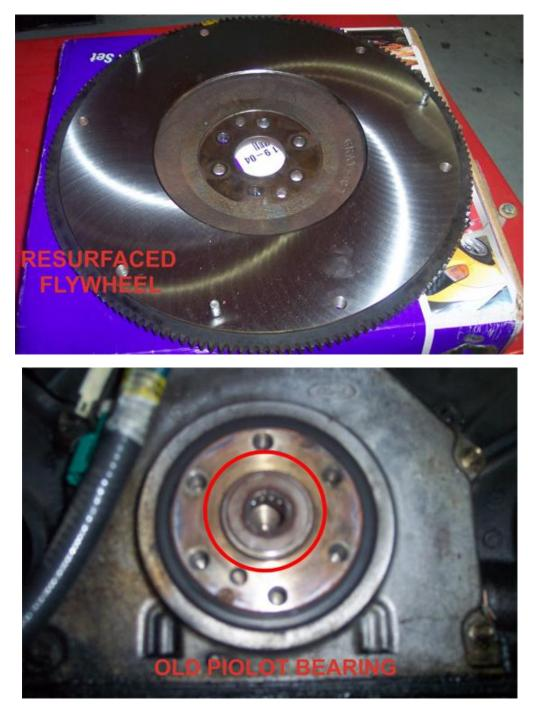
17. Now install your freshly resurfaced flywheel, line up the bolts and finger tighten them in a star pattern. They will need to be torqued to specs, when torquing the bolts torque them in a star pattern as well to prevent the flywheel from warping.
