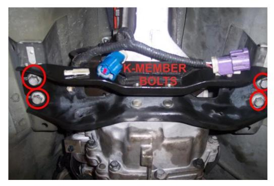
12. Next, slowly lower the transmission enough to get to the top two bolts, to remove them we used two 12in extensions, and two 6in extensions with a shallow 13mm socket on a wobble joint. After removing the top two bolts you can level the transmission back and remove the rest of the bolts 3 on one side, 2 on the other. 7 (13mm) Bolts total securing the transmission to the engine.
