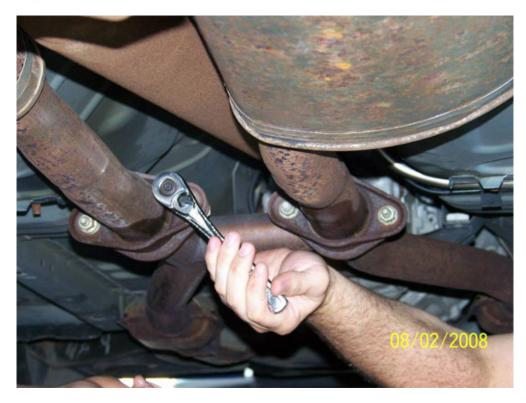
10. Put on your safety goggles and gloves if you have not already done so. Cut the factory exhaust as close to the center of the "hoop" that goes over the axle as you can. STEER CLEAR OF BRAKE LINES, FUEL LINES, etc.... In some cases, it may be easier to cut the exhaust in 2 or more places. The reciprocating saw will cut through the pipe in less then 30 seconds. Slide the exhaust from the hangers.
