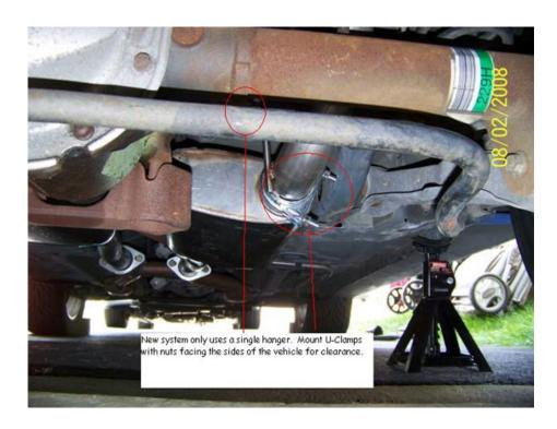
16. The new exhaust only has a single hanger, on the over-axle portion that uses the mount closest to the front of the vehicle/closer to floor boards.
