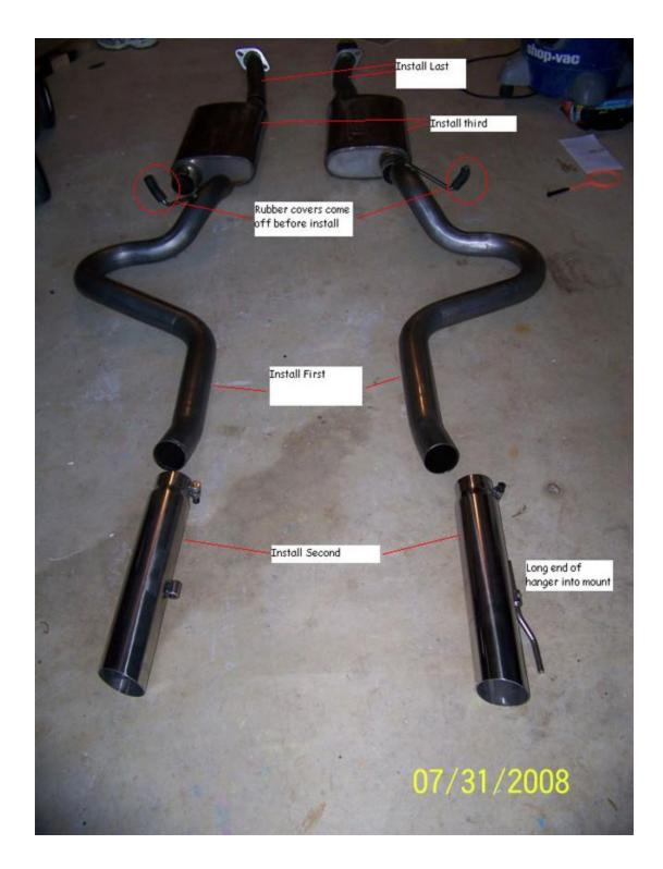
6. It may be necessary to file any rough edges off the tip of the hangers to ensure they fit properly (it was required during my installation). The machined Allen-Key clamps that hold these hangers do not allow for any deformities. The LONG side of the hanger slides into the mount.
