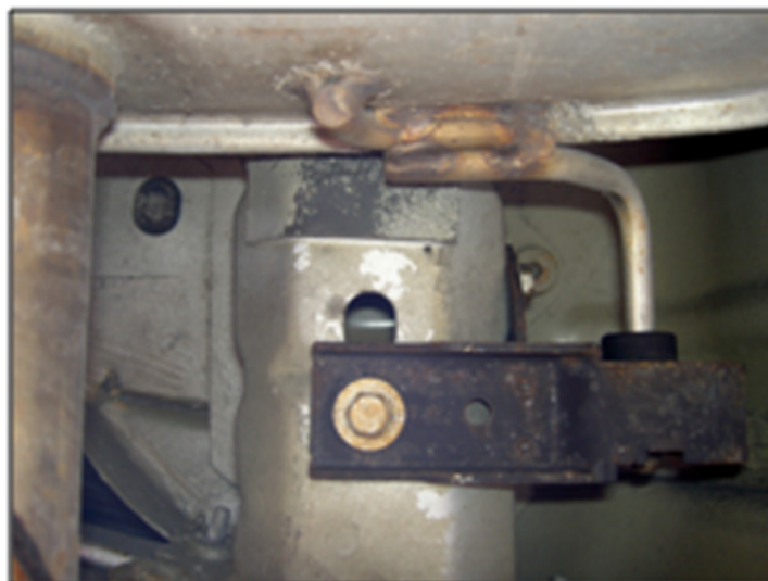
Figure 1: Depicting a metal muffler hanger bolted in place before installation.
