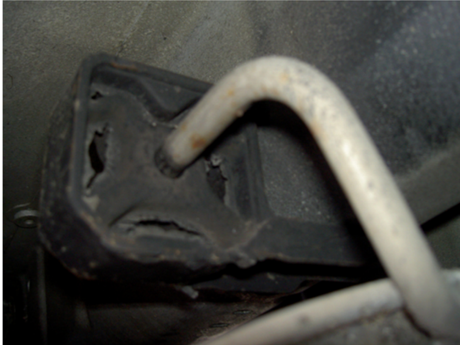
Figure 2: Depicting the rubber hole the muffler fits into.
