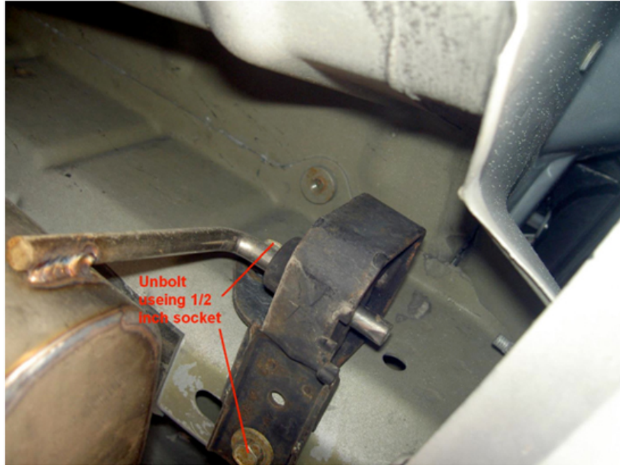
Figure 6: Depicting the last hanger with the TWO bolts that must be removed.
