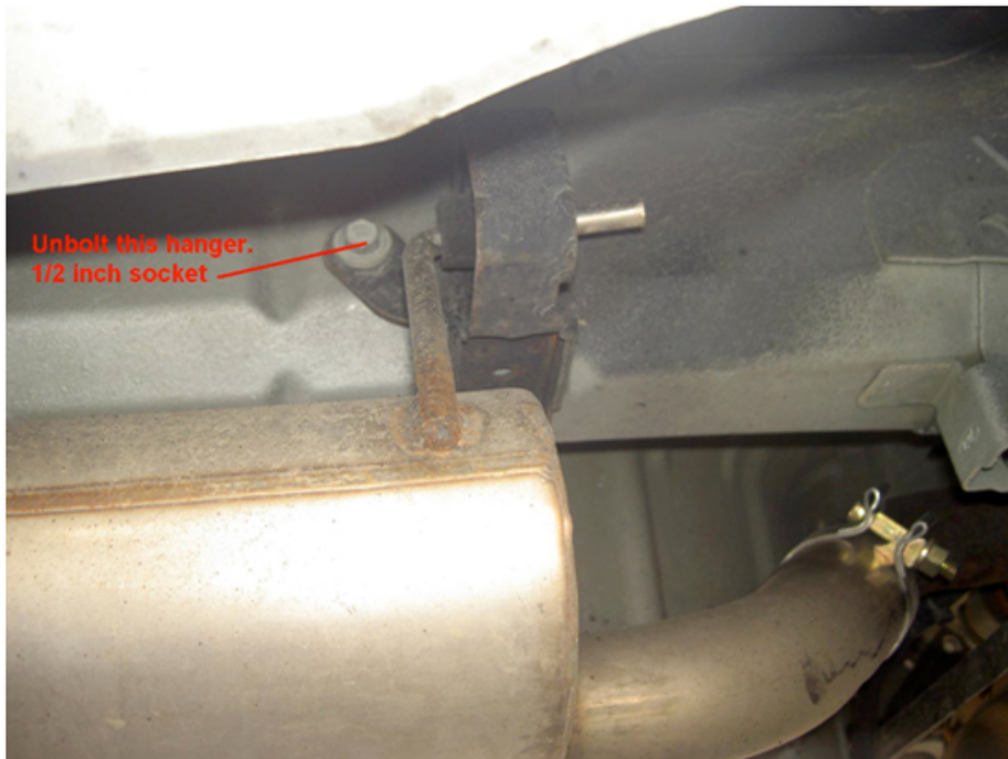
Figure 5: Depicting the hanger that is towards the mid pipe on the muffler with ONE bolt to remove.
