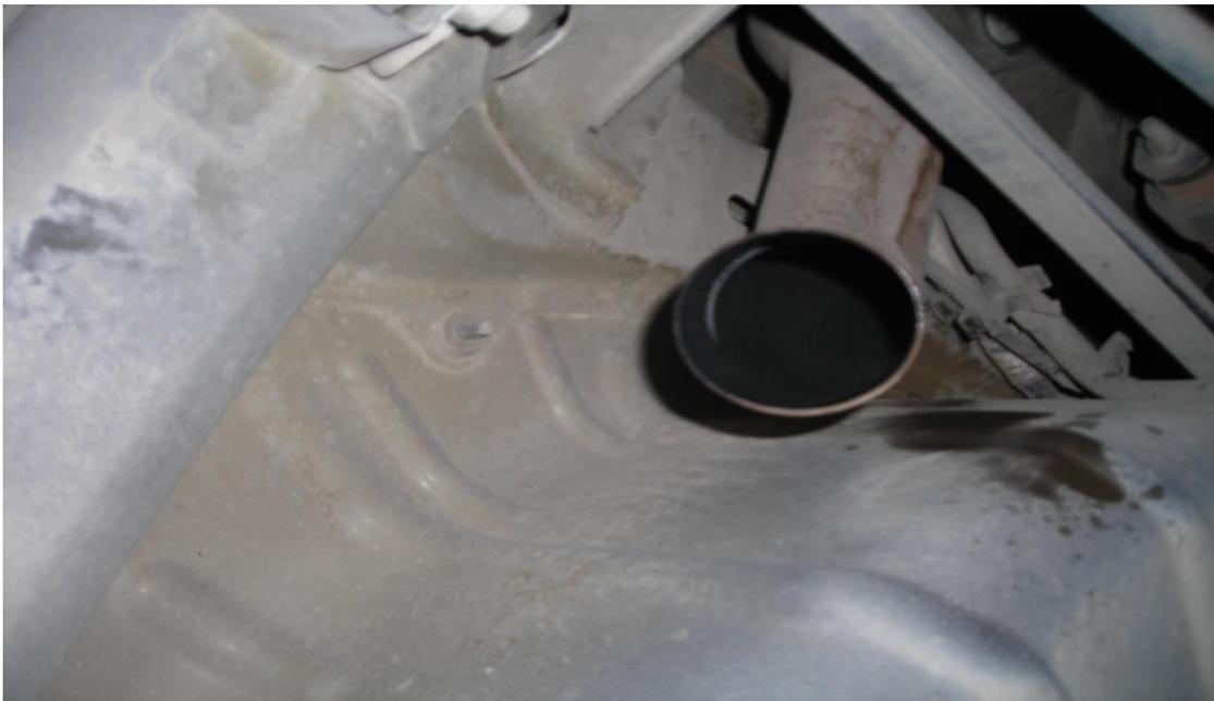
6. Slide the existing mufflers off of the mid-pipe to remove them.
