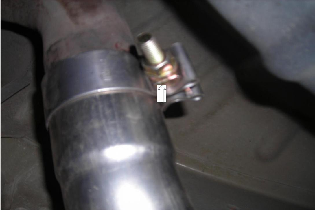
10. Tighten the bolt on the exhaust clamp that connects the neck of the Pype Bomb to the mid-pipe by using a 15 mm wrench
