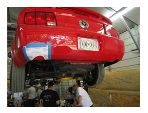
12. Once you have the template taped down in the correct place. Grab your precise air saw and start cutting. Make sure to leave roughly and 1/8" to a 1/4" between the paper and your cut. This way you can trim it back with a more precise tool.
