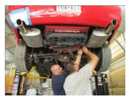
17. You may have to tap the holes for the universal mustang hangers on the driver's side. The hanger towards the front of the car will need an extra hole, and the hole won't be there. So, you can leave it hang, (which is just fine) Or, drill another hole.
