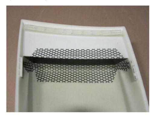
8. Once the grille is properly trimmed and fitted, remove it from the louver and thoroughly apply the supplied 3M Adhesion Promoter to both the surface of the louver where the grille will be applied as well as the grille itself. Cut two 6" strips and two 1" strips of tape from the supplied 40" role. After letting the Adhesion Promoter dry for a few seconds, place the tape strips as shown in the photo below.
