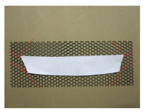
7. Test-fit the grille to the louver and make 90 degree bends as shown. At this point, if there is any excess material in the corners, you may trim it off so that the grille sits flush inside the louver.
