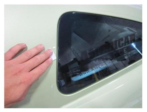
4. Peel the backing from the tape on the louvers and lightly place them on the vehicle in desired location. Make sure the louver covers the entire window and is parallel with the body line. Once they are in the desired location, press down firmly to fully seat the adhesive tape.
