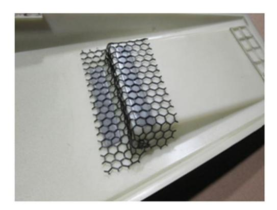
6. Lay the large grille on a flat surface with the supplied template sitting over top of it. Make cuts using tin snips as shown in the diagram below: These cuts leave a small amount of excess material in the corners that will be trimmed flush in the following step.
