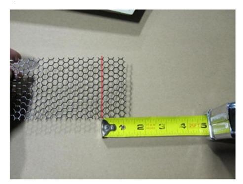
2. Make a 90 degree bend in the grille 1" from the edge as shown. Tip: Bending the grille on the edge of a table or workbench that is perfectly square ensures that you get a nice, straight edge.
