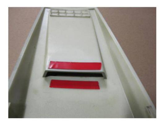
5. Remove the backing from the tape and place the grille on top of the tape as shown. Press down hard to fully seat the grille in the adhesive tape. Once the grille is in place, you may either cut the excess from the edges or simply fold them over as shown. These will not be seen when the louver is installed on the vehicle.
