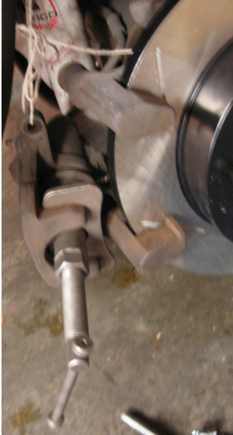
Brake compressor snugged onto piston.
