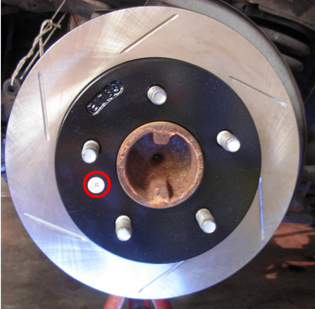
PowerSlot rotor installed on wheel hub. Notice the circled white "R" sticker is facing out.
