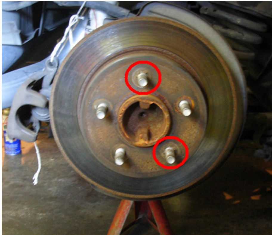
Wheel hub and rotor. Rotor retainers circled in red.
