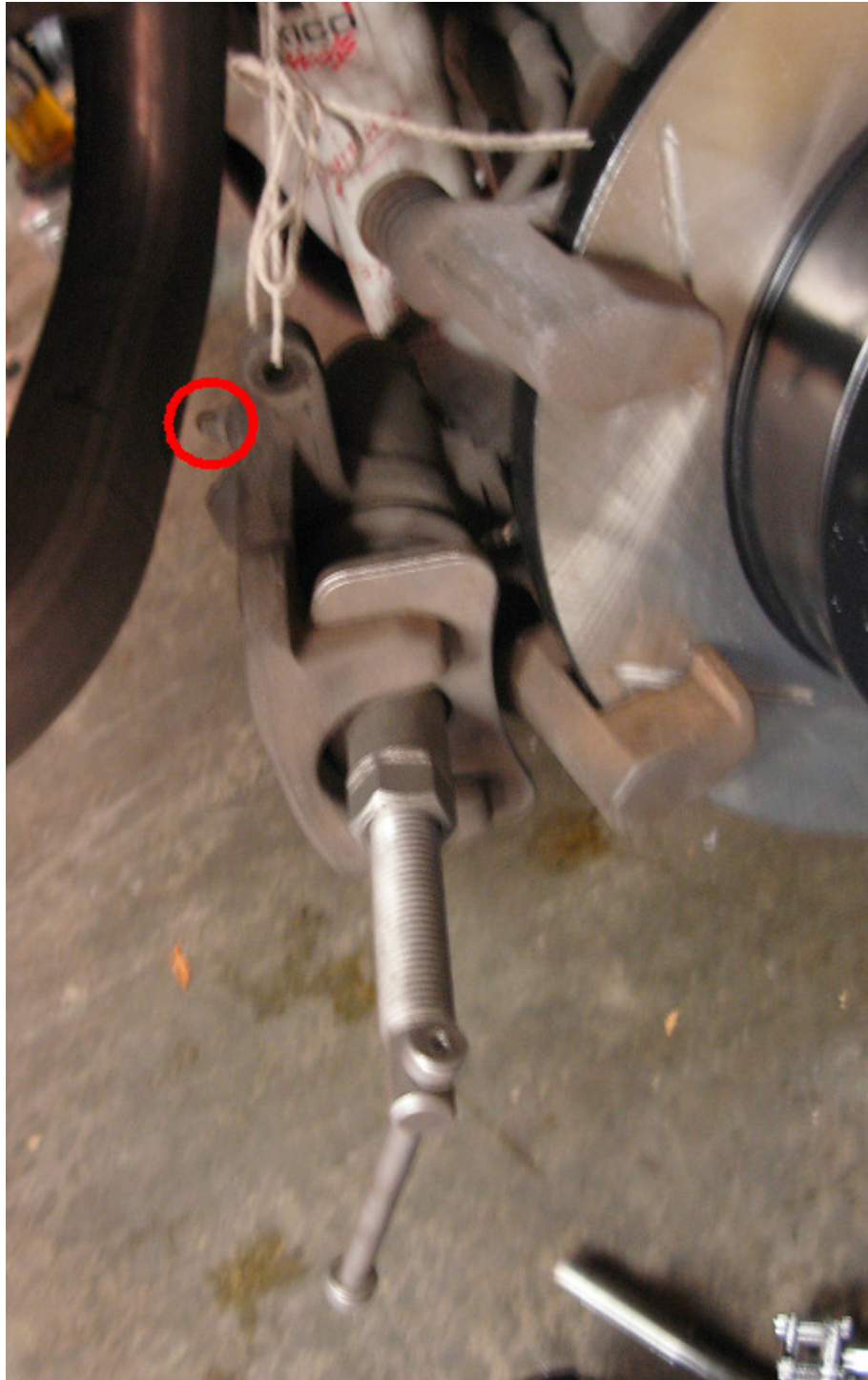
Brake caliper. The bleeder valve is circled in red.
