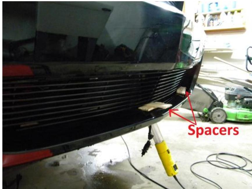
5. Locate the mounting tabs on your new grill and pre drill the hole. After your hole is predrilled begin to set the screw in but don't let it go too far. The locking clips should be set on the screw, as its peeking through the other side of the plastic and then the screw should be drilled in the rest of the way.
