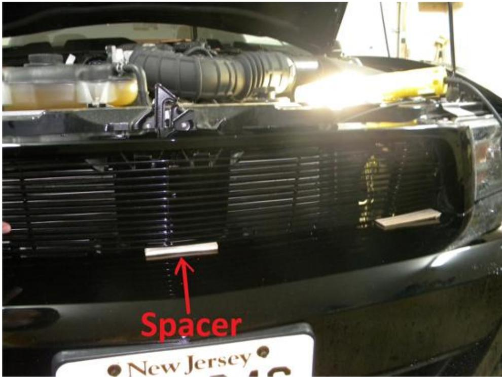
5. Locate the mounting tabs on your new grill and pre drill the hole. After your hole is predrilled begin to set the screw in but don't let it go too far. The locking clips should be set on the screw, as its peeking through the other side of the plastic and then the screw should be drilled in the rest of the way. This will allow for the locking clip to bind onto the plastic and hold the grille in place. Do this for all three mounting tabs.
