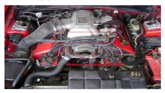
4. Now you will need to move the spark plug wires out of the way. You don't have to unhook them only move them away from the top of the alternator. You will also need to move the two vacuum lines that run across the top of the alternator. BE CAREFULL they break very easy!
