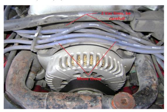
5. Now using the 3/8" drive ratchet, 6" extension and 10mm socket remove the alternator bracket. There are 2 bolts and 2 nuts that need to be removed.
