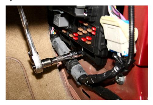
8. Pull the lower end of the Smart Junction Box towards the center of the car, and then once it's free pull the whole box down. The backside of the Smart Junction Box is where the One Touch Top Module is installed. So you may find it necessary to pull some of the surrounding wiring harness loose from the car to rotate the Smart Junction Box into a desirable position for you to access.
