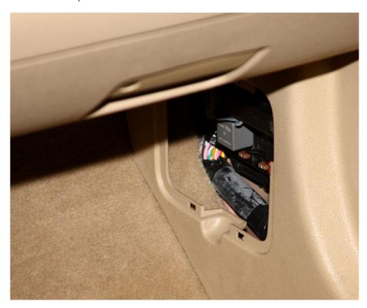
5. Remove the door sill trim plate by pulling up at its inner edge. The four clips (visible in the picture below) should pop loose with a little effort. There is also double-sided tape used to seal the plate to the body of the car. Once the clips have been popped loose, you can pull on the plate carefully, and the double-sided tape will separate from the car.
