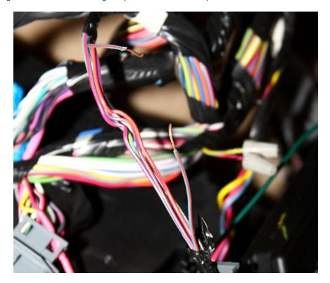
17. Connect the brown wire from the One Touch Top Module to the wire leaving the connector, and the red wire from the One Touch Top Module to the wire from the harness.
