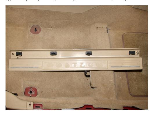
6. Next, remove the kick panel trim. It is held in place by four clips as well. You can see their locations in the picture below. It helps to have the square access panel removed, as it allows you to grip the kick panel a little easier. The lowermost clip will release by pulling the panel towards the center of the car, and the other three by pulling the panel towards the rear of the car.
