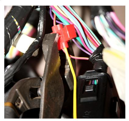
11. Next find one of the black wires, and use a quick-splice connector to connect the green wire of the One-Touch Top Module to it. Once the quick-splice's tab is pressed in, snap the plastic cover into place.
