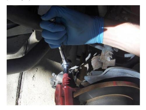
5. After loosening the top bolt, take the 12mm hex wrench to loosen the bottom bolt from the rear of the caliper. (there is not enough room for the socket for this step.) You may need a pair of pliers to hold the connector from spinning while loosening the bolt.
