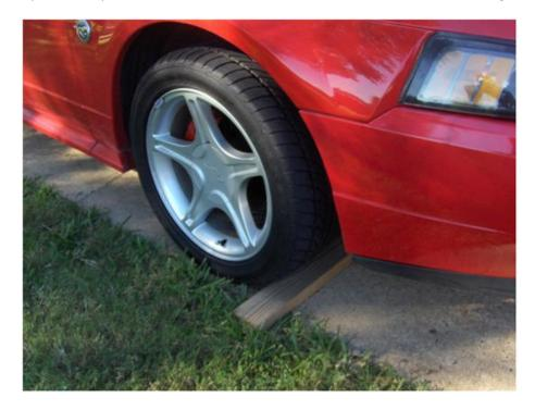
2. Next it's time to pop off the center cover of your wheel and loosen the lug nuts (do not remove them) before lifting the car off the ground. After loosening all the nut it's time to lift the car slowly off the ground high enough to place a jack stand securely under, then slowly lower the car onto the jack stand in a suitable position.
