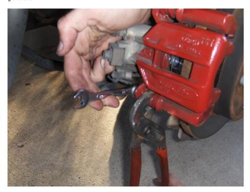
6. Now that both bolts are loose, remove both bolts and gently remove the caliper by pulling it straight up being careful not to bend or pinch any of the brake lines. Warning! In this step, you will be removing the caliper, make sure to have a way to secure it up in the wheel well in such a manner that the line is not stressed.
