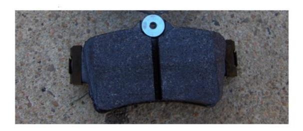
\*\* IMPORTANT INSTALLATION NOTE\*\* Never apply any grease to this surface of the brakes. This surface should remain as clean as possible and should have nothing added to it, under any circumstances \*\*
