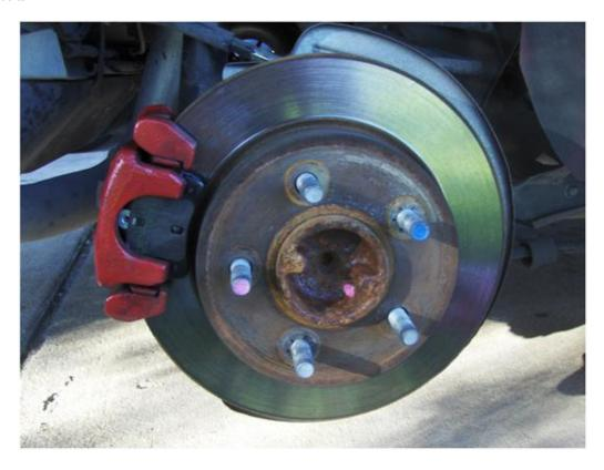
12. Now that everything is back in place you can reinstall the wheel and snug the lug nuts into place. Next slowly lower the car back onto the ground. Then evenly tighten up all the lugs in a star pattern and replace the center cover.
