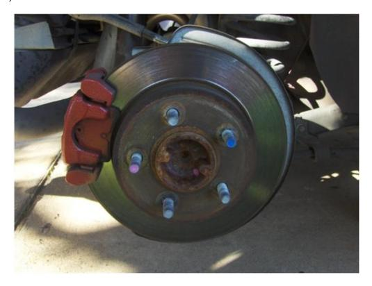
4. Using a 12mm socket began loosening the top bolt located on the backside of the caliper (do not completely remove the bolt until you remove the bottom bolt). Leaving the top bolt in will make it easier to loosen the bottom bolt without the caliper moving on you.
