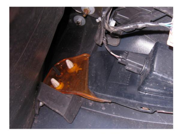
11. Once both clips are released simply push the turn signal assembly towards the inside of the car and the inner retaining tab will release the light assembly.
