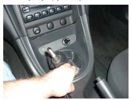
3. Using a 10mm socket, unscrew and remove the stock shifter handle.
