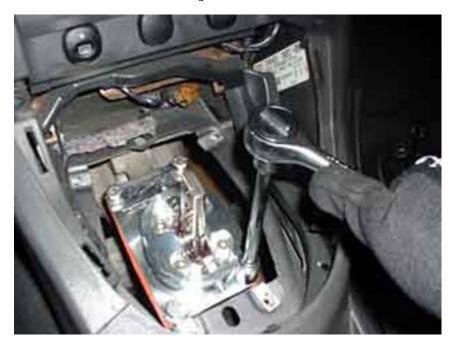
13. Set the shifter stops in strict accordance with Steeda's instructions. The stop bolts and jam nuts can be adjusted with a 1/2" wrench. **Tip:** To get a good look at the space between the shift lever and stop bolts, shine a flashlight downwards behind the lever. You should be able to see a sliver of light between the lever and the stop bolt, which should disappear once you put pressure on the lever. Slide the boot washer over the shift lever once the stops are adjusted.
