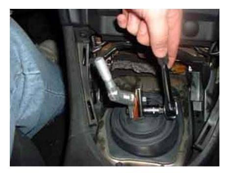
17. Plug the cigarette lighter back in, and slide the boot cover back over the shifter handle. Press down firmly to resecure the cover on the console.
