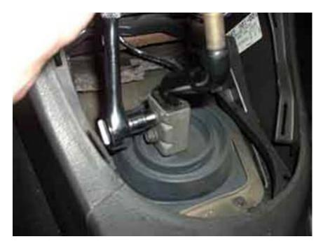
4. Unscrew the four bolts from the cover plate using an 8mm socket with an extension.
