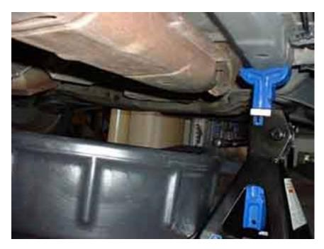
Royal Purple Synchromax is a high-performance manual transmission fluid that will complement the short-throw shifter by allowing the smoothest possible operation of the transmission. The T5 takes 5.6 pints, or 2.8 quarts (check your car's owner's manual). That means three bottles will be necessary for this fluid change.
