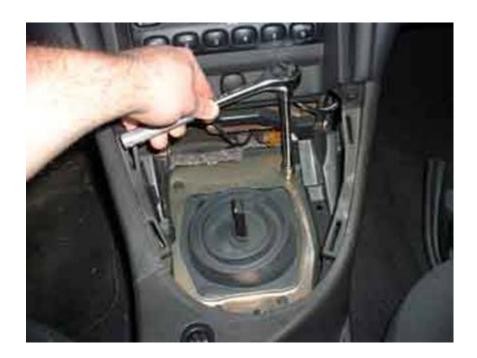
5. Using a 13mm socket and extension, remove the four bolts holding the stock shifter on the transmission.
