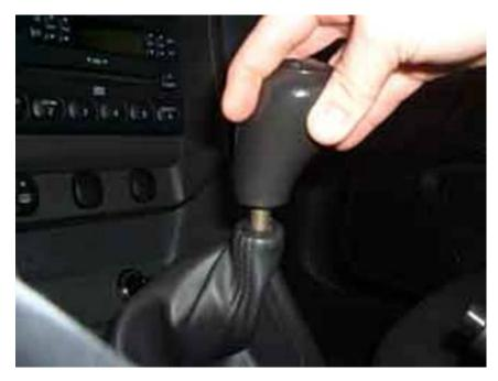
2. Pull the cover off the shifter and unplug the cigarette lighter plug. It's easiest to do this by grabbing around the shift boot and pulling (see illustration). Check to make sure the clips stay on the tabs on the edge of the cover; I had one fall onto the inner boot. Tuck the cigarette lighter's plug out of the way.
