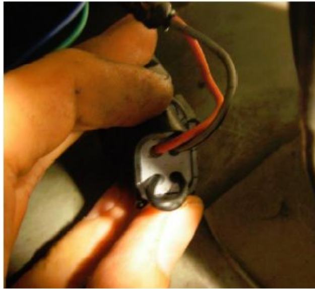
Rear of connector shell with VSS vehicle harness wires installed.
