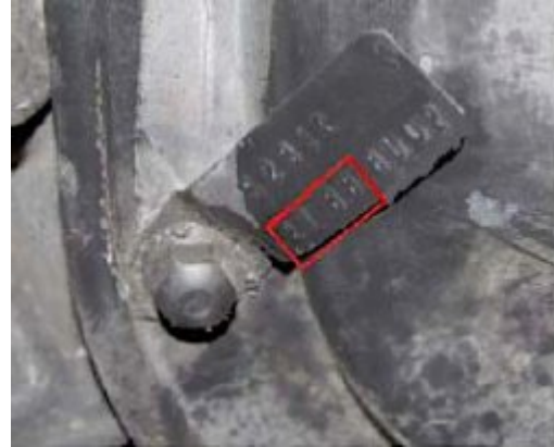
Tag numbers used to determine gear ratio.
