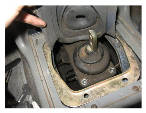
7. Lift the old shifter out of the way. This may require some force as the old silicone is still holding it to the transmission. Be careful trying not to let dirt or dust fall into the transmission.
