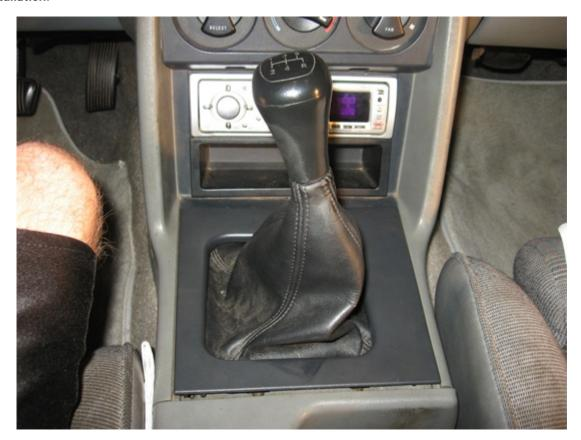
1. Remove shifter knob by twisting it off.
