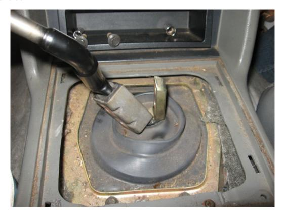
5. Use the 8 mm socket wrench to remove the two visible bolts retaining the metal ring around the second shifter boot. Then use an 8 mm wrench to remove the two bolts securing the front of the metal ring. This may take a while, unless you want to remove the whole console. If you don't remove the console, you will need to use the needle nose pliers to remove the staple holding the rubber boot to the metal retaining ring. You will then be able to move the rubber boot out of the way when necessary.
