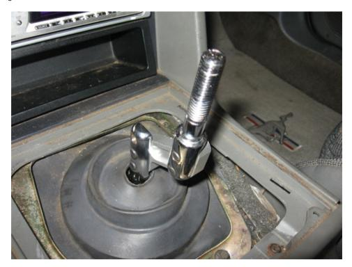
15. Replace leather shifter boot over new shifter and reinstall the shift knob.
