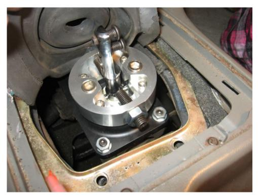
13. Again, verify that the shifter shifts it through all the gears properly. Reinstall the rubber boot over the new shifter and fasten the ring using the four, 8 mm bolts removed earlier, making sure the rubber boot is secured properly.
