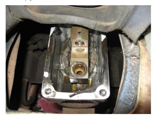
8. Use the razor blade to fully remove the old silicone to prepare the surface for the new shifter.
