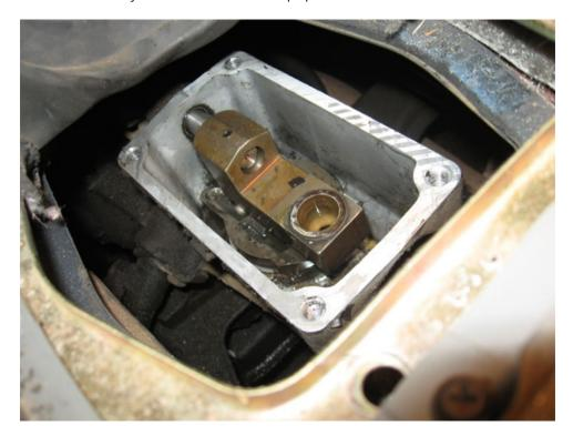
9. With the 4 mm Allen wrench, attach the four screws to the transmission in preparation for the new shifter. Make sure they are tight.
