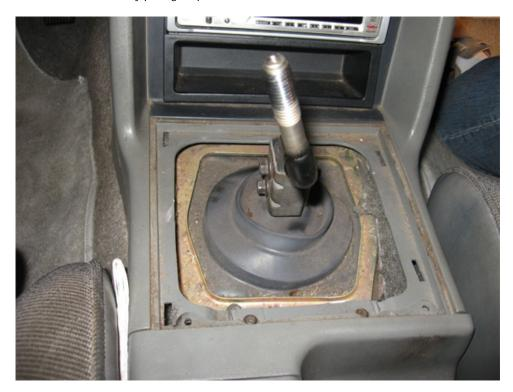
4. Using the 10mm socket, remove the two screws attaching the shifter handle to the shifter and remove the old shifter handle.
