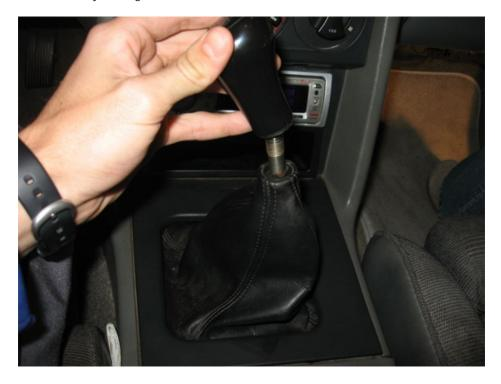
2. Remove shifter console trim, which should pop off with a bit of force. Make sure the metal clips are attached to the 4 tabs for reinstallation.
