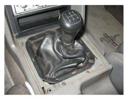
16. Snap the shifter console trim back on and you're done. If you have time, however, you may want to wait to give the silicone proper drying time, as instructed by silicone package (usually about 24 hours if possible).
