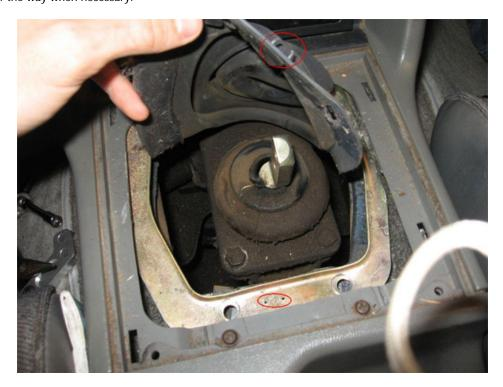
6. Now you have access to the shifter. Use a 13 mm wrench and/or socket wrench to remove the 4 bolts securing the shifter to the transmission.
