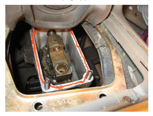
12. Position the new shifter on the screws already installed, which will make attachment simple. Push the new shifter all the way down and attach the four, 14 mm nuts until tight.
