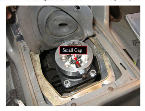
11. Remove the shifter and apply a bead of silicone all the way around the surface, to be bonded to the transmission as shown Be sure to follow instructions on silicone package for proper use.
