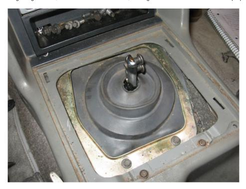
14. Using the 5 mm Allen wrench and the screws provided in the kit, attach the new shifter as shown. When attaching the new handle, select the height you want, as the new kit has two height settings, as shown in the height comparison photo earlier. Use the top two holes for the medium height or the bottom two holes for the low height setting.
