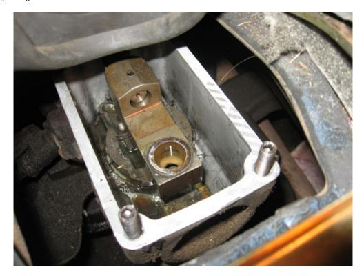
10. Set the new shifter in to check fitment. Using the 6 mm Allen wrench, adjust the screws included with the kit so that when the transmission is in gear, there is only a small gap between the shifter and the end of the screw (~1/16"). Then fasten the nut to hold the screws tight. Also make sure the transmission shifts through all the gears as it should.
