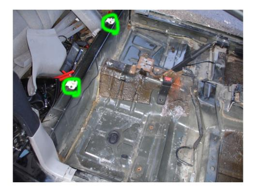
14. You can finally pull up that ugly, stained carpet. You can rip it right out, or you can roll the front towards the back and try to collect as much dirt and dust as you can as you pull it out.
