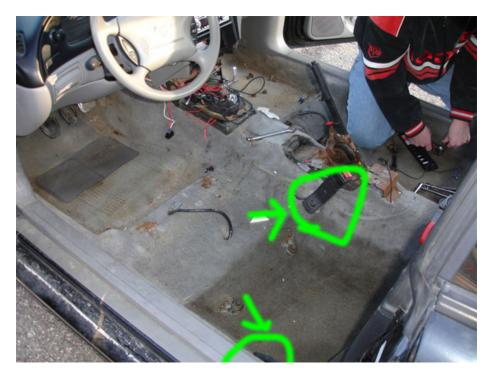
11. Start taking out the trim at this point. The door sills pull straight up and off. They may need some persuasion from underneath with a screwdriver because there are metal clips that hold them down and they can be very hard to let loose.
