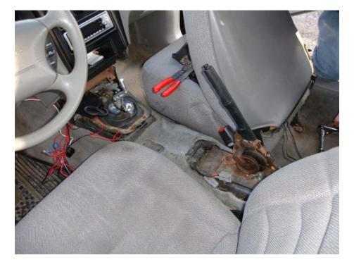
9. The hard part is done and you can take out the seats. There are two bolts on the front of the track and also two on the back. They are both 15mm. Take the four out and lift the seats up and out. If they are electric seats, make sure to disconnect any electrical wires before yanking the seats out.
