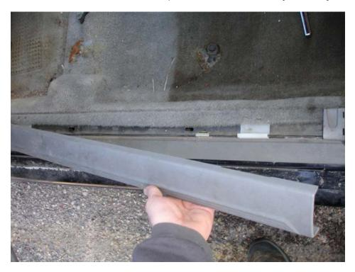
12. You can then pull the kick panels from each side. There is one plastic push pin on each one, and if you can get your hand up and underneath the kick panel, it will pull straight out with a little force.
