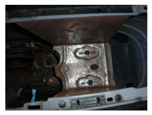
8. Now this gets tricky, taking the center console out. I found it easiest to pull the console a little towards the back and then tilt the back end up. While doing this, either your or a friend should disconnect the wires for your fog lights, and also the cigarette lighters, if applicable.
