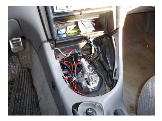
5. Next, pull out the center console cubby. There are two screws holding it in, and they are covered up with some rubber pieces. Then pull upwards on this and it will pop right up and out.
