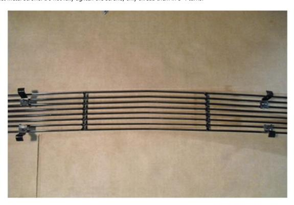
4. Place the billet grille over the factory grille. From underneath the car, adjust the J-Hooks to wrap around the factory plastic grille as shown.
