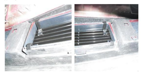
5. Once all of the hooks are secured around the factory bumper, use a Phillips head screwdriver to tighten the screws from the front of the vehicle.
