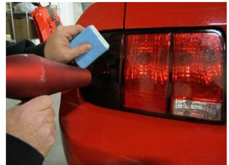
*Note from 99-04 put the bottom piece on then the piece that sits on top the brake light. Making sure the first is dry and cooled before doing the second. Then heat the top and with your hands wet roll the top over the bottom.*
