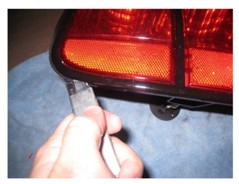
2. Slide a screwdriver under the trim to remove the part of the trim that is between the lights going slow and making sure that you are careful not to break the trim.
