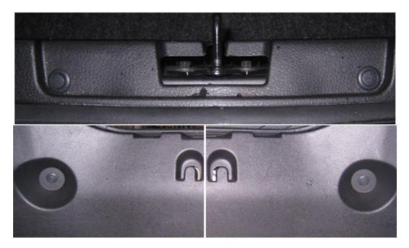
3. While slightly tugging the outer end of the plastic center piece unscrew the plastic clips. This will put tension on them allowing you to unscrew them without damaging the clips. (recommended method)
